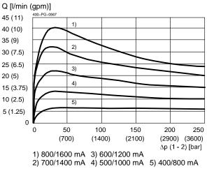
$\Delta p = f(Q)$  Pressure drop - Flow rate characteristic [MDT32GS...-24]
