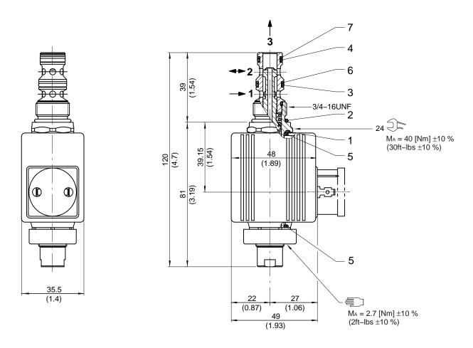
6.2 Option with emergency override pin "P" and option with emergency override "S"
