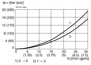
Q = f (I;  $\Delta p$ ) Flow rate adjustment characteristic [MDT32GS...-24] – 1 → 2 with constant pressure drop Q [l/min (gpm)]
