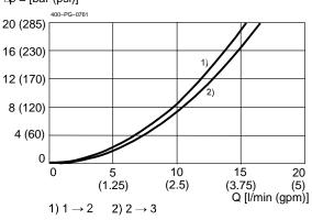
Q = f (I;  $\Delta p$ ) Flow rate adjustment characteristic [MDT32GS...-10] – 1 → 2 with constant pressure drop Q [l/min (gpm)]
