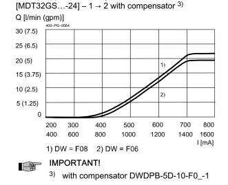
Q = f (I;  $\Delta p$ ) Flow rate adjustment characteristic
