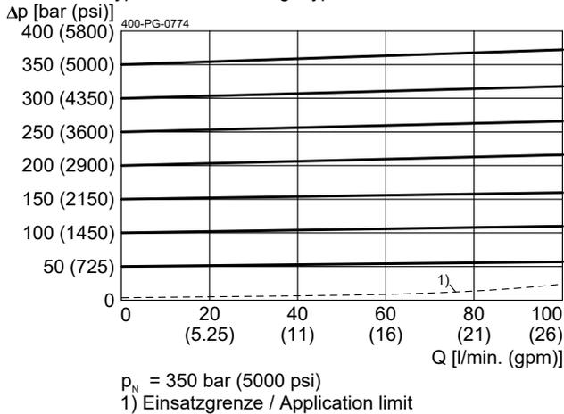
$\Delta p = f(Q)$  Druckverlust-Volumenstrom
