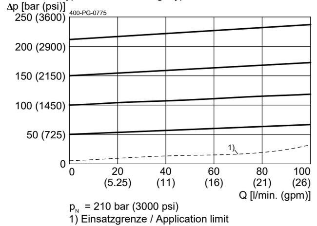
$\Delta p = f(Q)$  Druckverlust-Volumenstrom
