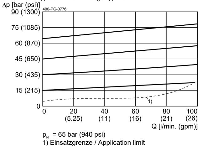
$\Delta p = f(Q)$  Druckverlust-Volumenstrom
