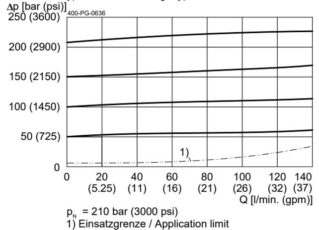
$\Delta p = f(Q)$  Druckverlust-Volumenstrom
