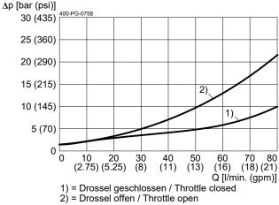
$Q = f(I:\Delta p)$  Flow rate adjustment Adjustment, normal opening Measured with supply channel 1 and 2 = Ø0.28"
